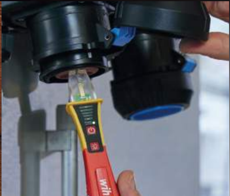
Internationally adjusted measurement tip for all sockets around the world
