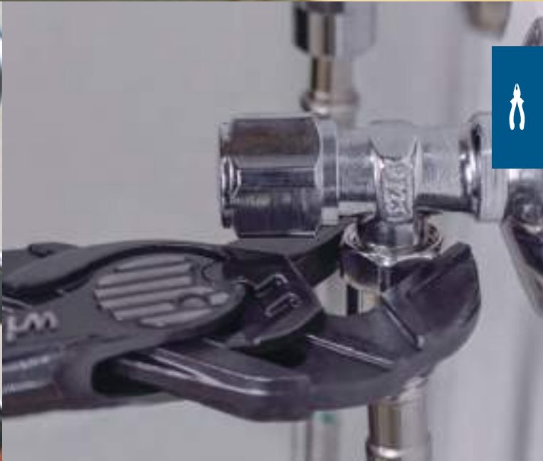
Quick fastening thanks to the ratchet function
